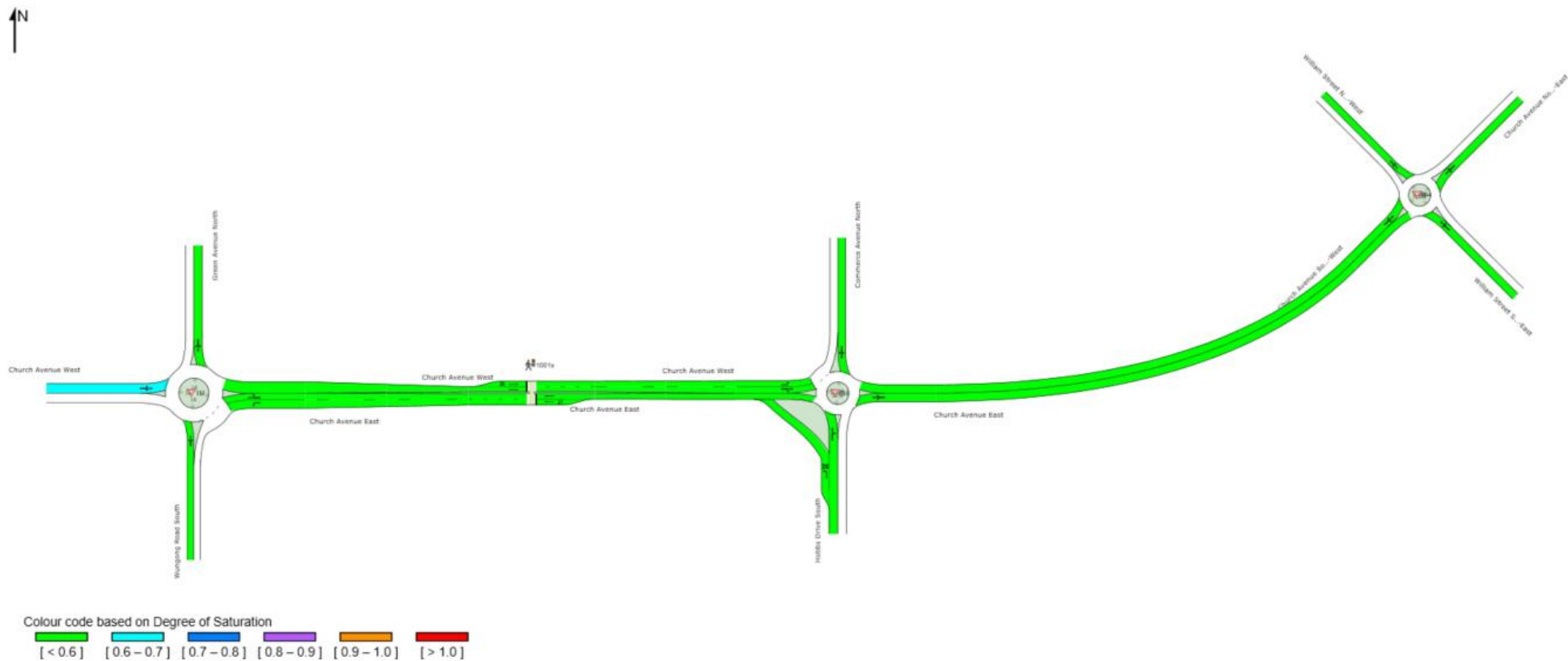
Figure 5.23 Degree of Saturation - Church Avenue Road Network – AM Peak - Do Nothing Scenario (LX at grade)
