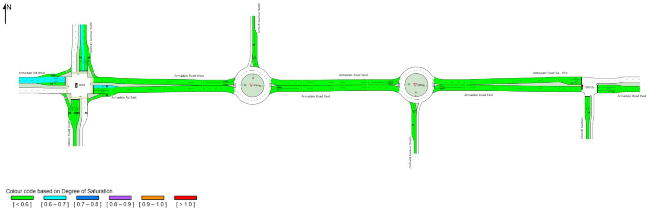
Figure 5.20 Degree of Saturation - Armadale Road Network – Do Something Scenario (grade separated) – Partial treatment – AM Peak
