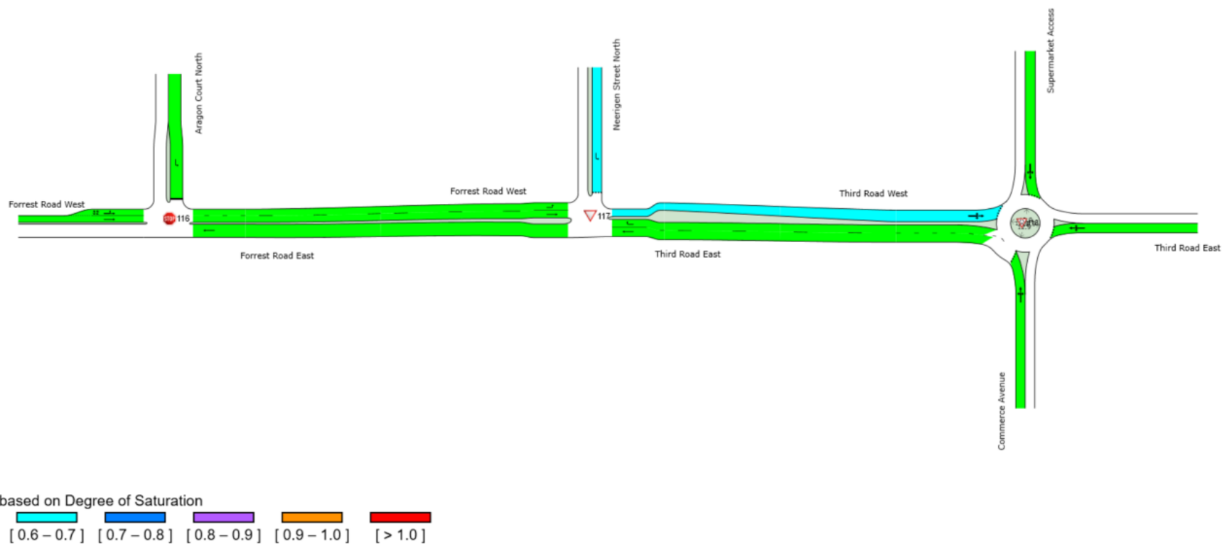
Figure 7.33 Degree of Saturation - Forrest Road Network – PM peak - Do Nothing Scenario (grade separated)
