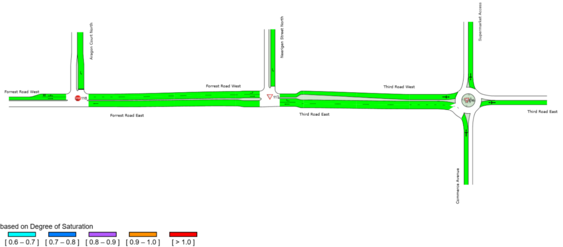
Figure 5.33 Degree of Saturation - Forrest Road Network – PM peak - Do Nothing Scenario (grade separated)
