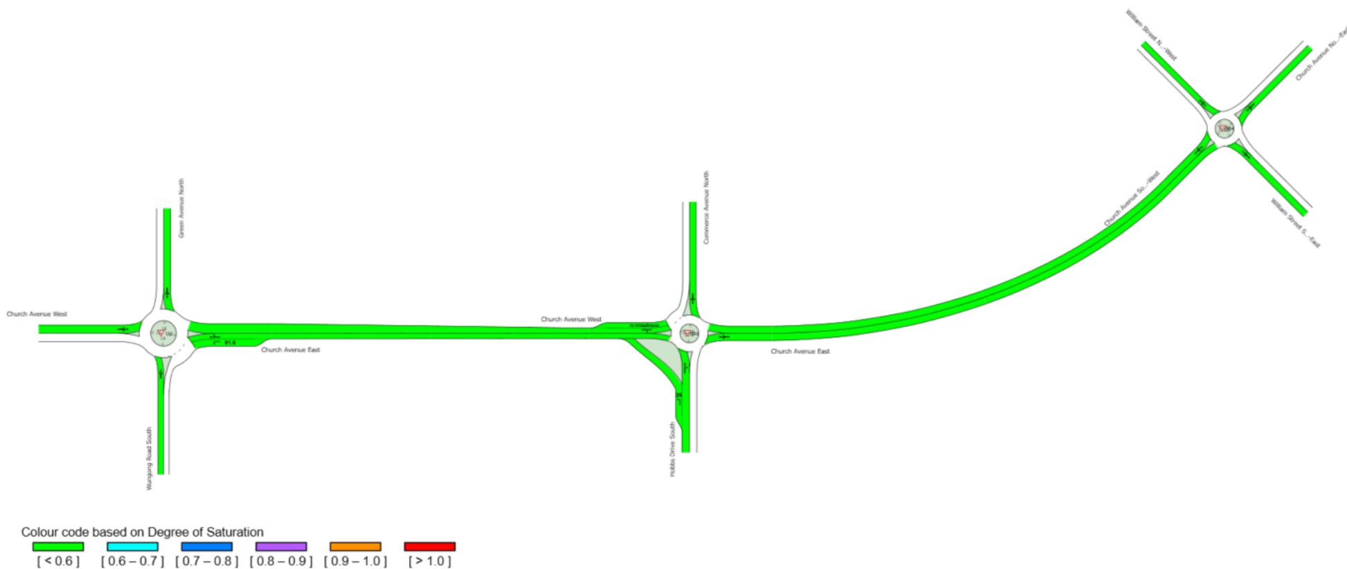
Figure 5.27 Degree of saturation - Church Avenue Road Network – PM Peak - Do Nothing Scenario (grade separated)
