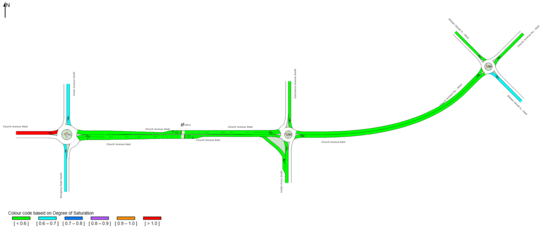
Figure 7.23 Degree of Saturation - Church Avenue Road Network – AM Peak - Do Nothing Scenario (LX at grade)
