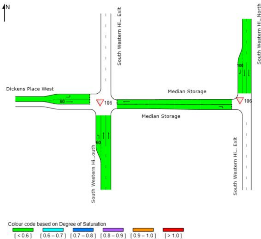
Figure 4.9 Degree of Saturation -SWH/ Dickens PI – AM Peak - with SWH duplication
